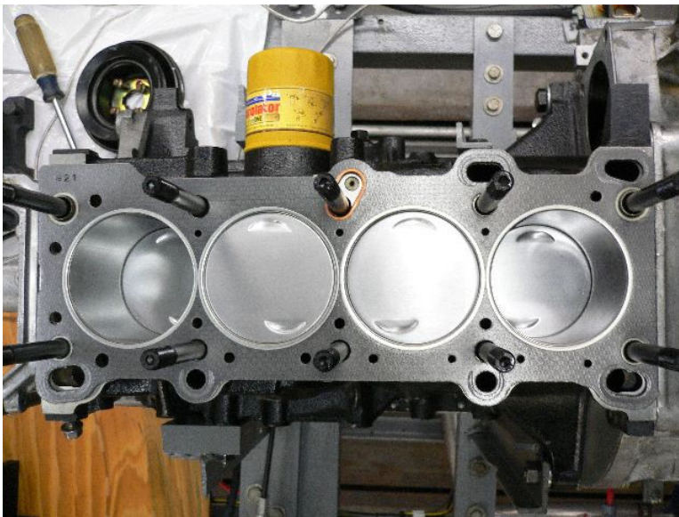
Figure 3 - Short Block with Flat Top Pistons
