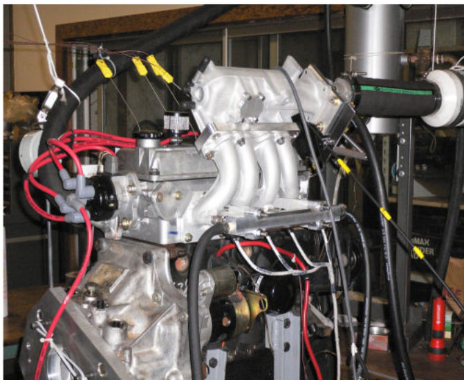
Figure 14 - Engine setup with Port Fuel Injection
