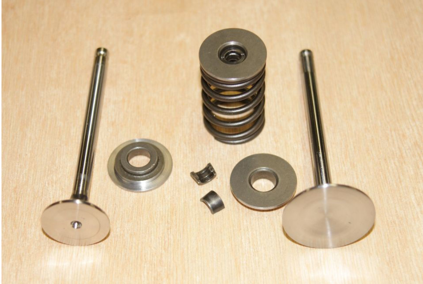
Figure 6 - SHS Valves, springs and retainers
