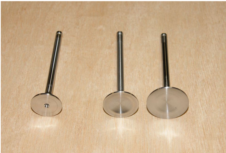
Figure 5 – Valves, Pictured Left to right Exhaust Valve, LS and HS Intake Valve, SHS Intake Valve
